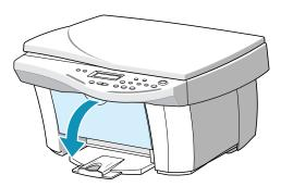
**2** After the print cartridges have moved to the centre of the product, unplug the power cord to turn the power off with the cartridge holder in the centre.
